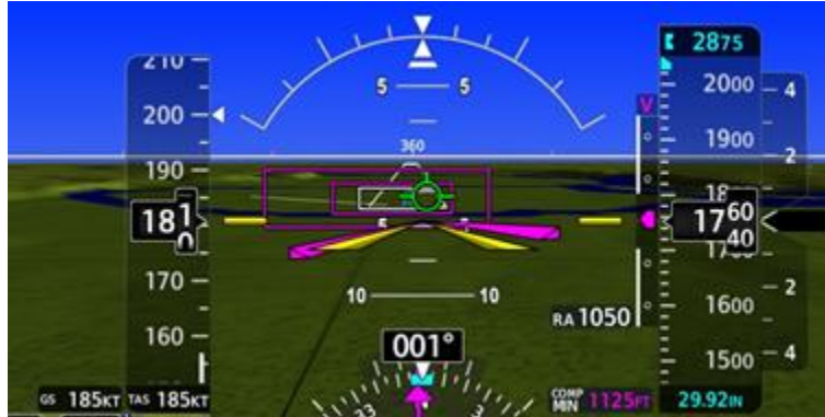
Figure 8, Vertical Deviation Display With Barometric Approach Vertical Guidance
