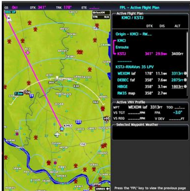
Figure 5, Display of Temperature-Compensated Altitudes
