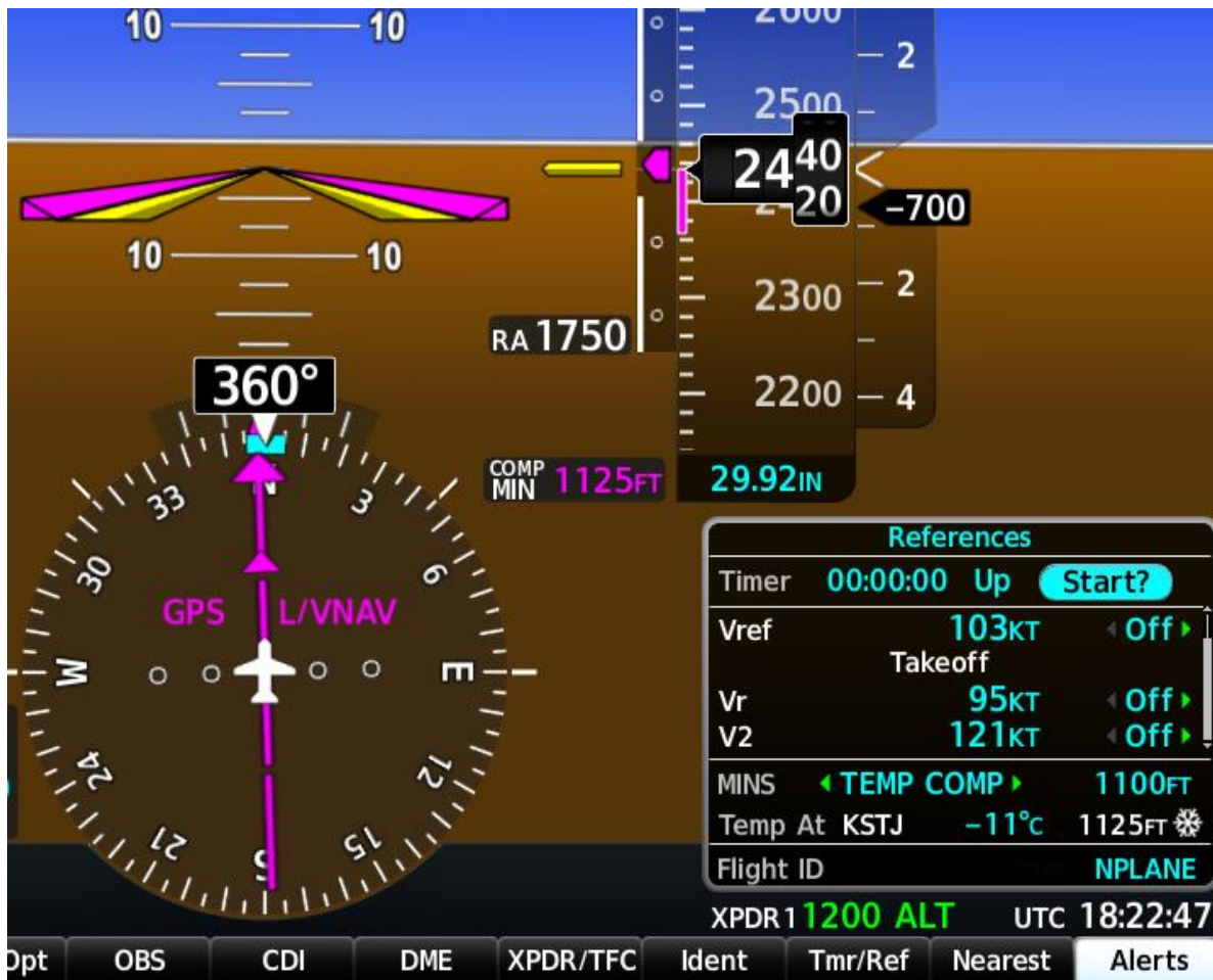
Figure 6, Temperature Compensation of Minimum Altitude
