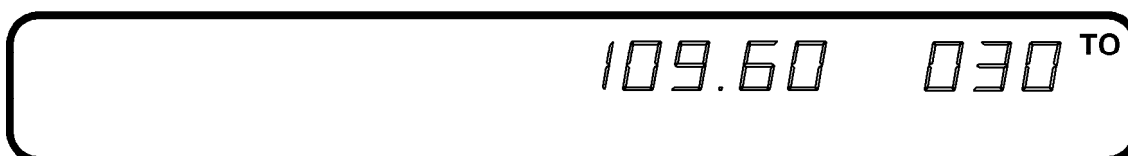
VOR MODE: ACTIVE "BEARING TO" FUNCTION DISPLAY
